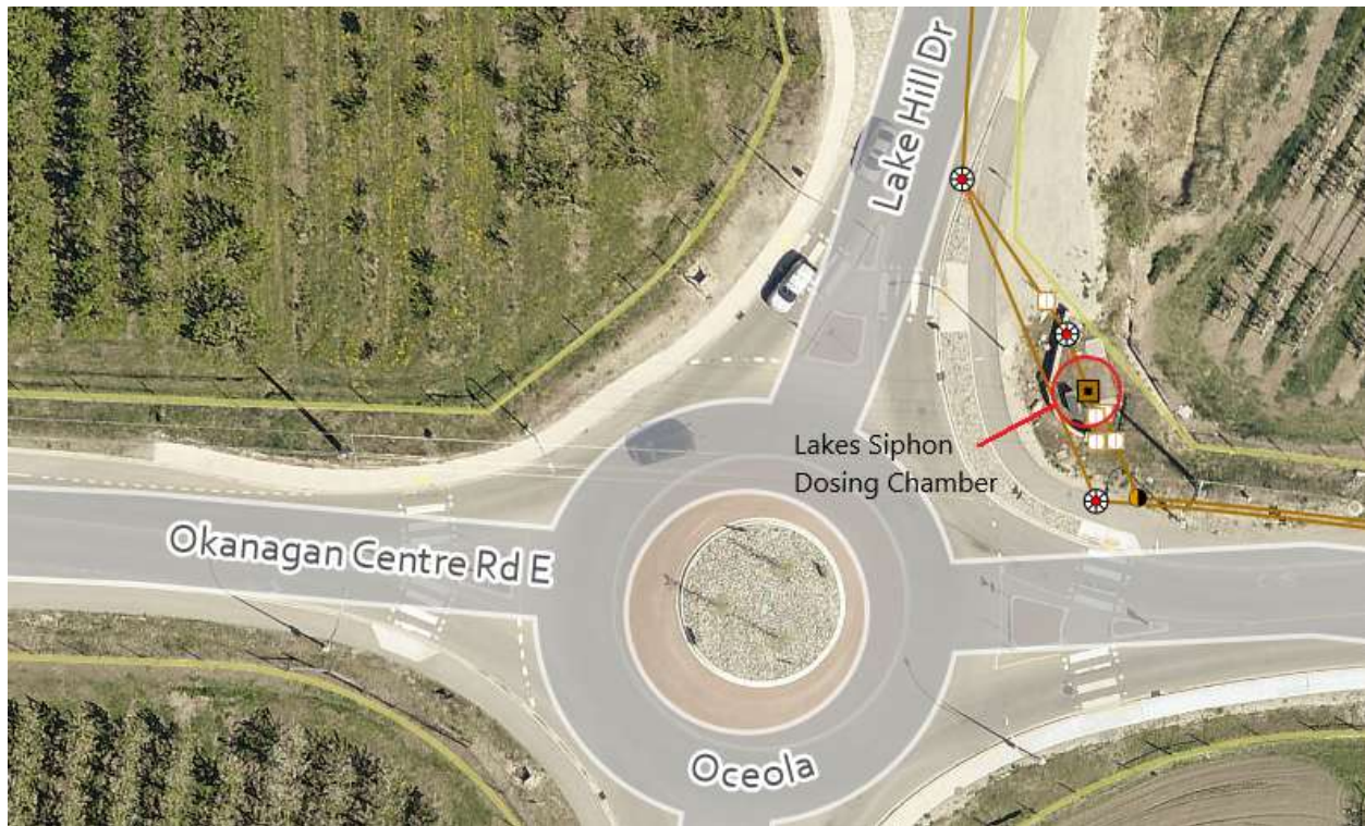
Figure 2: Lakes Siphon Dosing Chamber
