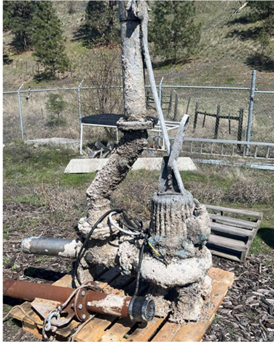
Figure 3: Old TWAS Aerator
