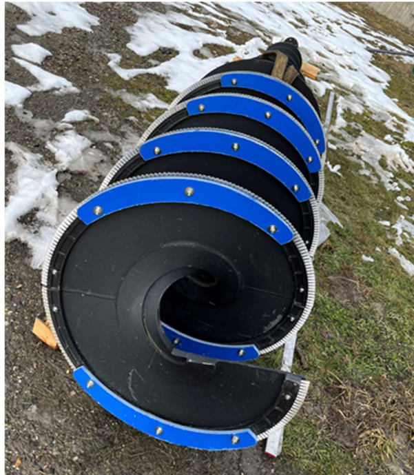
Figure 4: New Septage Auger Screen
