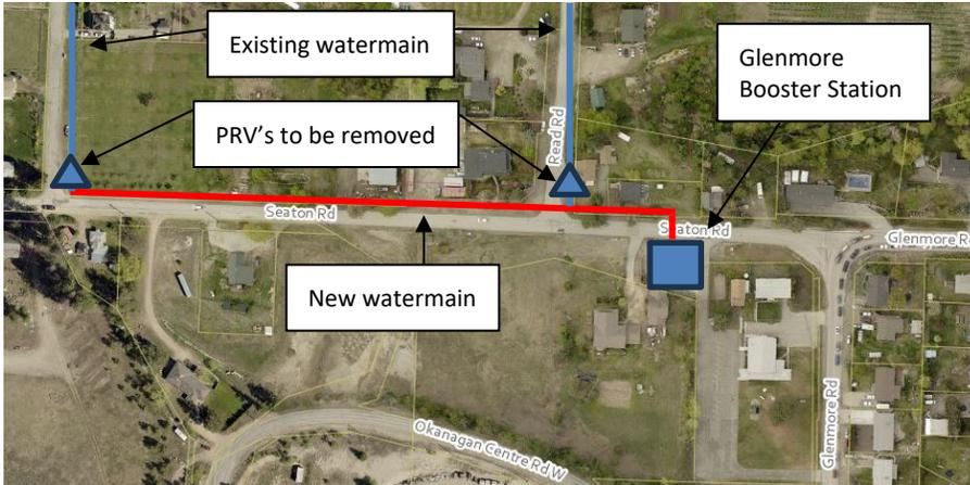
A recent analysis of the distribution system identified that the two pressure regulating stations can be effectively removed if water is supplied from the Glenmore Road pressure zone. Removal of these two stations will reduce operational costs, eliminate future replacement costs, and eliminate a confined space hazard.
