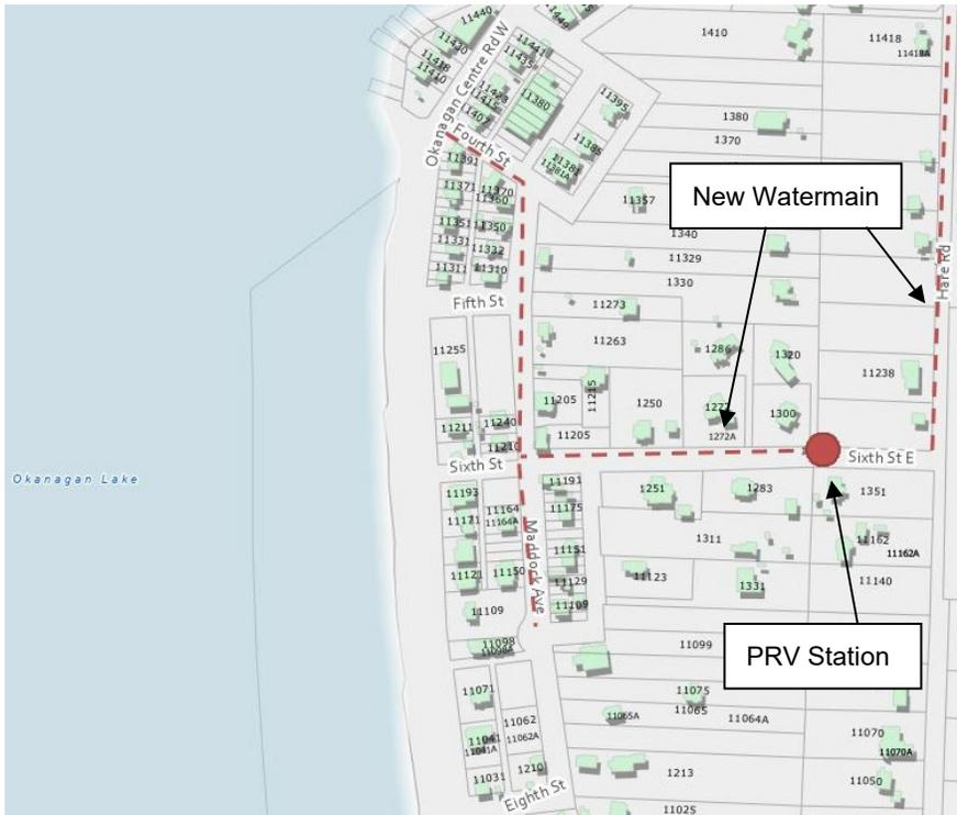
In 2022 the watermain on the south end of Hare Road, and part of Sixth St, was replaced and upsized. This was done with the goal of increasing fire flow and replacing aging infrastructure.
